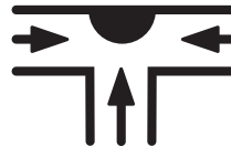
180° Half Dome for 3-Way "T" intersections
