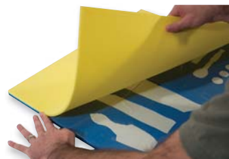
Align foam layers to adhere adhesive backing.
