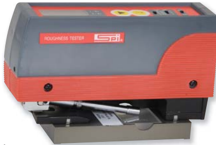
Roughness tester placed on standard for calibration.
